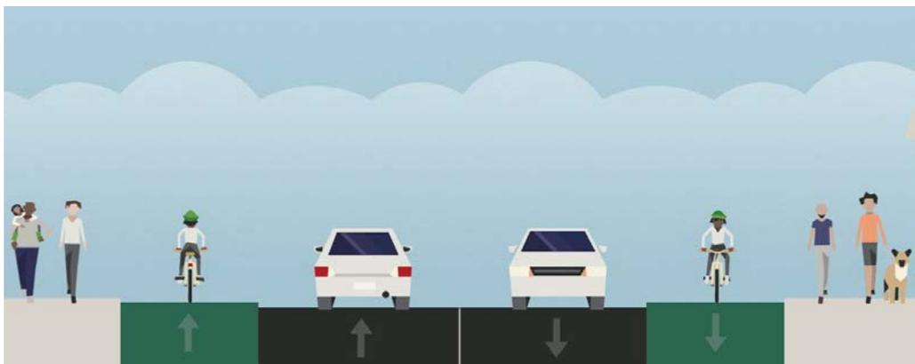
*Stepped cycle tracks are vertically separated from the footway and main carriageway*
