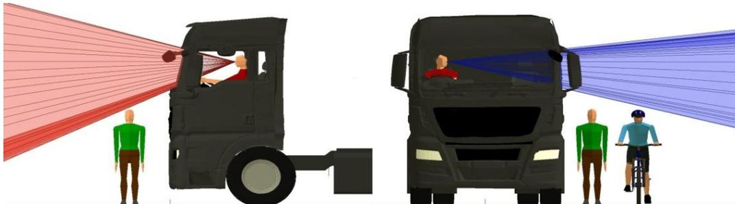
**Fig. 2: Example of direct vision enabled by a standard N3G cab**
